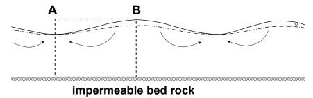
Flow lines symmetrically converge at A and diverge at B.  $\rightarrow$  A and B are considered impermeable boundaries.
