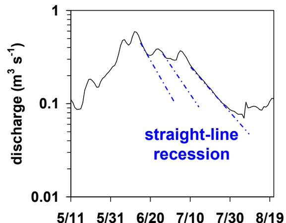
Recession hydrographs commonly plot as straight lines on a semi-log graph.
