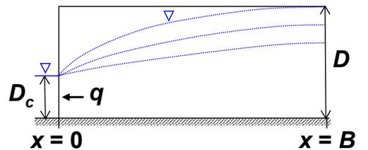
Approximate analytical solution is obtained by 'linearizing' the Boussinesq equation:
