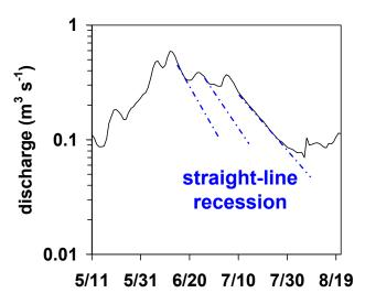
Recession hydrographs commonly plot as straight lines on a semi-log graph.
