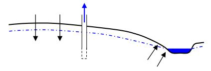
Recharge - Discharge - Pumping = Storage Change (water level ↑↓)
