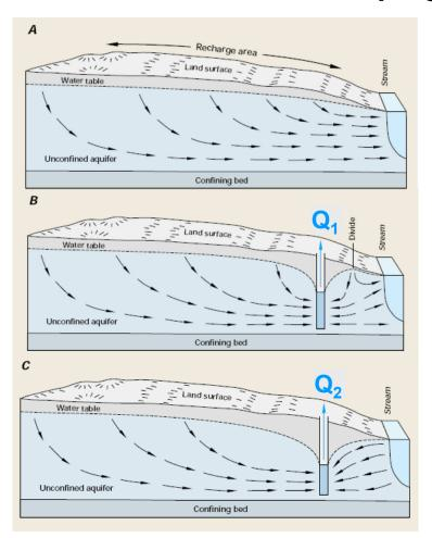
GW discharges to the stream under undisturbed conditions.
