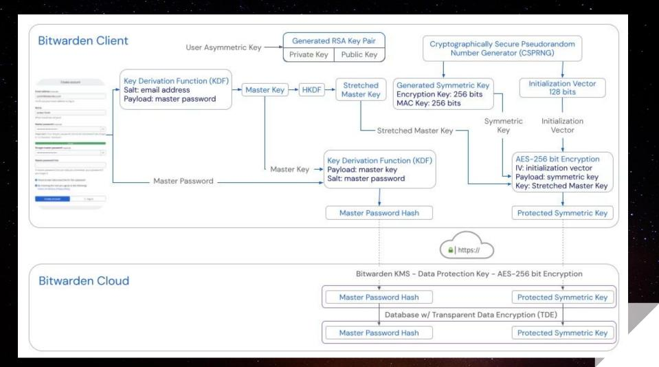
Finally, the Stretch Master key and Protected Symmetric key (AES-256) are used to decrypt vault items (usernames and passwords)
