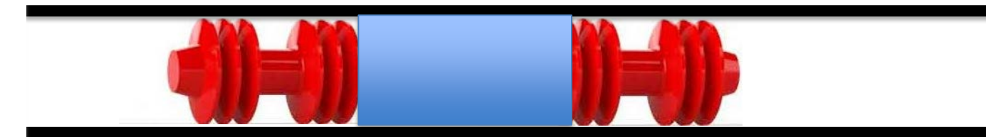
Chemical Batch Pigging
