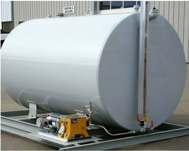
Inhibitor and Biocide Injection
