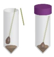
**6.** Break the top of the swab handle so that the length is below the top of the tube. Close the tube with the lid, ensuring that the lid is seated/sealed well. The broken end of the swab handle can be discarded.
