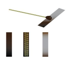
**5.** Immediately insert the swab into the conical tube that contains the preservative, and swish around to make sure the preservative contacts the sample material.
