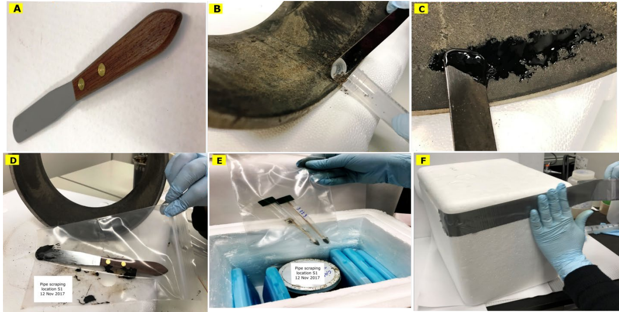
Figure 9: Representation of steps to be followed for collecting solid samples for Microbiological Analysis and MI-UDC Testing. (A) Use the sterile sampling spoon provided in the kit as shown in the picture, (B) Scrape the surface of the pipe using the spoon, and collect as much sample as possible into the sterile tube; label tube on the side and on the cap of the container, (C) Using a separate sterile knife repeat step (B) for any additional sludge adhered to the pipe's surface, (D) Transfer spoons used for sample collection into Ziploc bags and label the bag, (E) Transfer the Ziploc bags containing the knife and the tubes into an insulated container and place the ice packs, (F) Seal the box on all sides, stick a sheet with the box details on top /side of the box and send it for shipment
