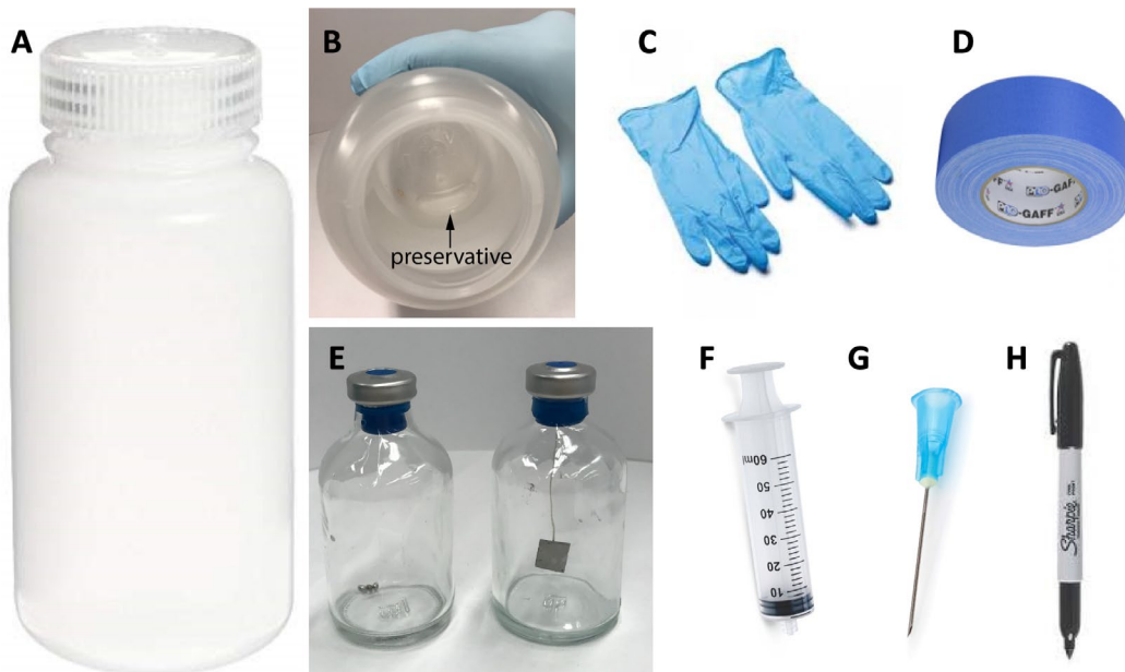
Figure 1: Supplies for liquids sampling. (A) 1-L Nalgene bottle, (B) 4ml preservative already added to the Nalgene bottle and should not be discarded , (C) latex/nitrile gloves, (D) labelling tape, (E) glass serum
