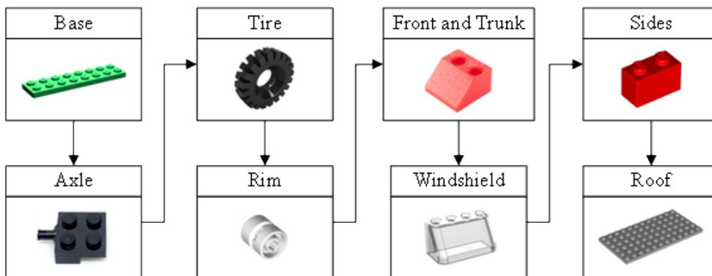
Figure 4. Processes for car toy assembly [19].
